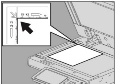
Place your sheet face down with the corner against the top left corner of the scanner and close the scanner top.
