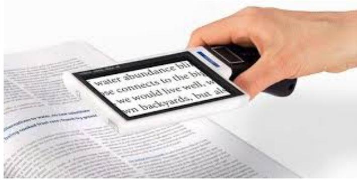
Portable digital magnifiers have a camera on one side that you hold over what you are trying to read, the magnified image is displayed on the other side of the monitor. They come in a number of different screen sizes as a separate device or are also available as an app on your smartphone. Some portable video magnifiers can also connect to your own computer or laptop so that you can angle it in different directions to see something like a board or projector screen in a classroom.
