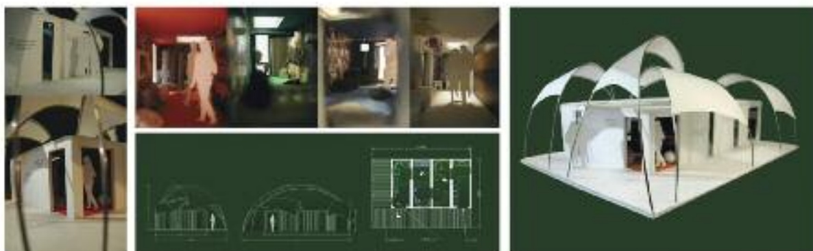
A mobile exhibition pavilion to showcase the U.K. and Ireland's finest contemporary eco-design has been created using discarded shipping containers. Visitors enter via the plastics display and through to timber and paper, to metal and fabric and finally to an information and events area. Facts and figures based on waste associated with these materials are displayed internally and externally. (Design Competition in the field for Design Competition, 08)
