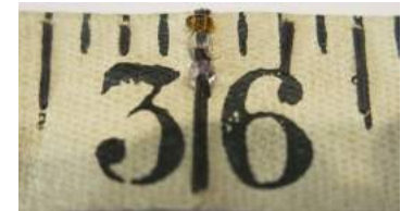
Figure 9.2. Detail of tactile tape measure showing beads added to indicate yard measurement
